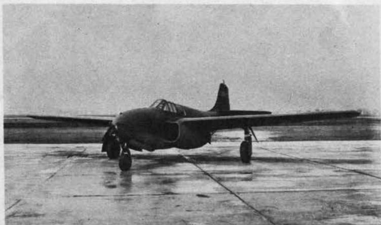
Bulky jet units are located beneath the P-59A's midwing, snug up against the fuselage. They give plane its distinctive broad, shallow fuselage which, when seen head-on, is its best recognition feature.
